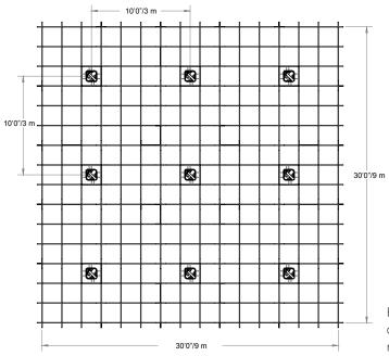
Example placement of 4000 lumen fixture on a 9' / 2.74 m ceiling, achieving 30 FC / 300 lux task plane luminance and 250 melanopic equivalent daylight illuminance (m-EDI).
