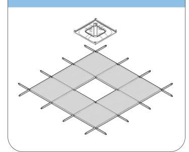
**STEP 2** Fold out t-bar clips over the ceiling grid structure & connect safety wires through safety wire slot.
