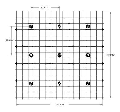
Example placement of 4000 lumen fixture on a 9' / 2.74m ceiling, achieving 30 FC / 300 lux task plane luminance and 250 melanopic equivalent daylight illuminance (m- EDI).
